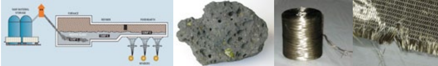
Basalt fiber basic manufacturing process Basalt rock raw material Spun Basalt fiber Basalt fabric
